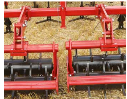
Advantages of self-cleaning roller with spikes
