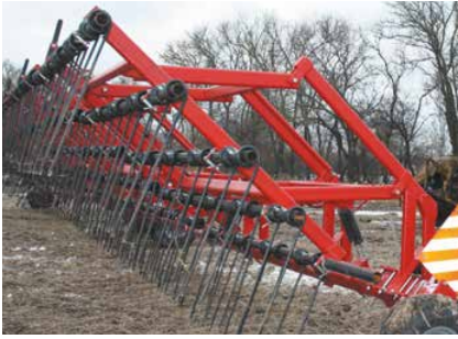
Suspension of work sections
