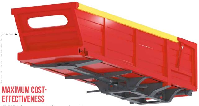
KELT XXL has no separate frame and consists of integral body with mounted elements of chassis and pivoting bogie, which provides sufficient durability with low weight.
