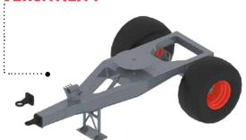
Trailer and pivoting bogie are joined by means of standard bolster, which enables to transport trailer by tractor trucks and to use pivoting bogie for this purpose.
