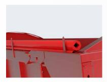
All trailers (except of trailers with screw conveyor and additional sides) can be equipped with manually-driven protective cover. Folded cover is fixed on the left side.
