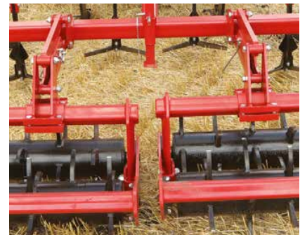
Advantages of self-cleaning roller with spikes
