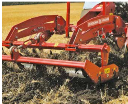
Balancing mounting of roller
