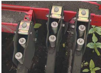
Two-stage adjustment of pressure
