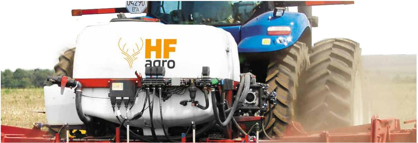
The SHILLING can be equipped with an additional HF Agro module for applying basic and starting liquid fertilizers simultaneously with the main operation of the unit.
