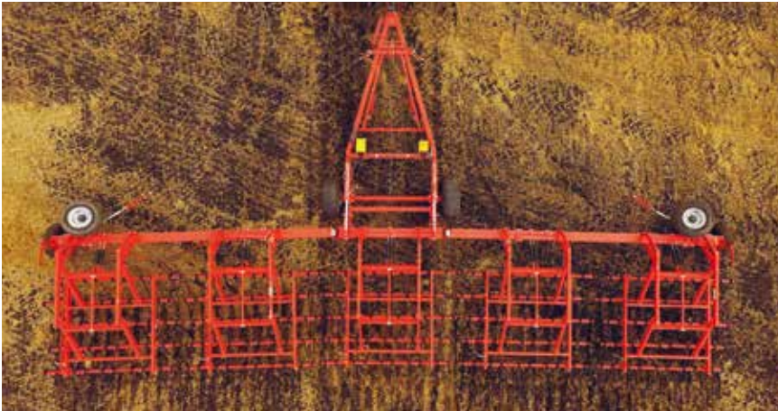
Cable tightening of sections
