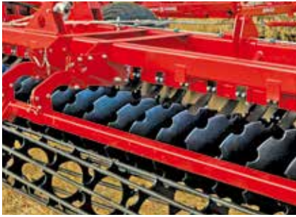
Roller maintenance-free bearing unit
